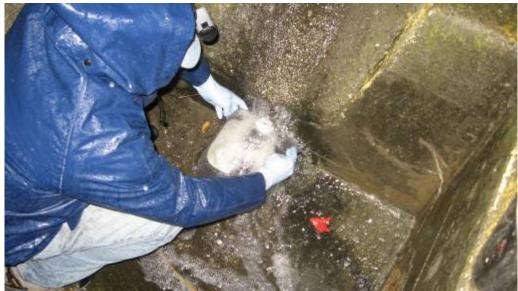
Collecting a sheet flow stormwater sample.
